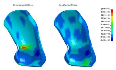
Figure 1. Typical stress distribution along the circumferential and longitudinal direction of ascending aorta and pulmonary autograft.
